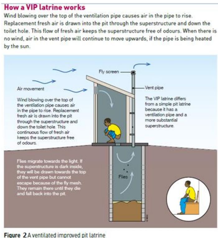
Fig 2: Ventilated Improved Pit - Loughborough University UK
